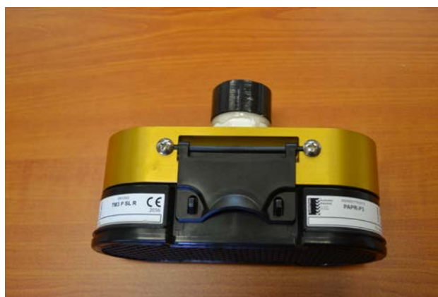
Figure 3.3 Example of custom made adapter to mount filter inside the Experimental Chamber
